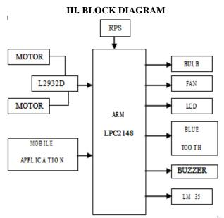
Fig 3.1:- Block diagram of prototype
