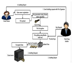
Fig 4.1.1: Overall Architecture of the System.
