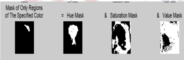
Figure 4.6 Applying Threshold Ranges
