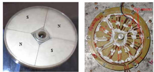
Figure 5: Flywheel Recessed With Permanent Magnets
