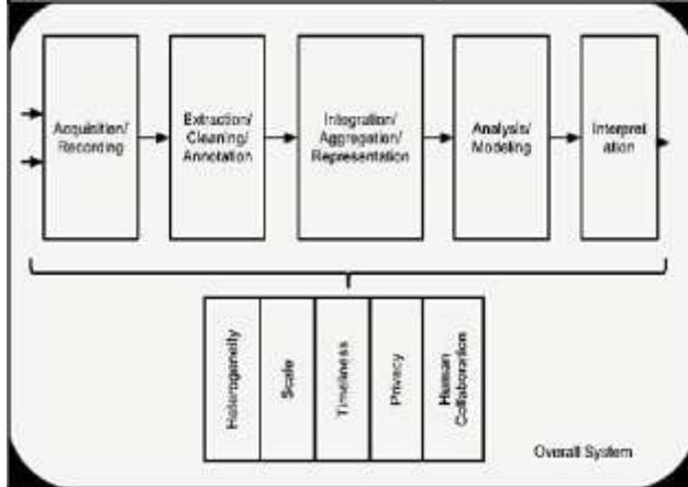
**Fig. 1: The Big Data Analysis Pipeline. Major Steps in analysis of big Data are shown in the flow at top. Below it are big data needs that make these takes challenging**
