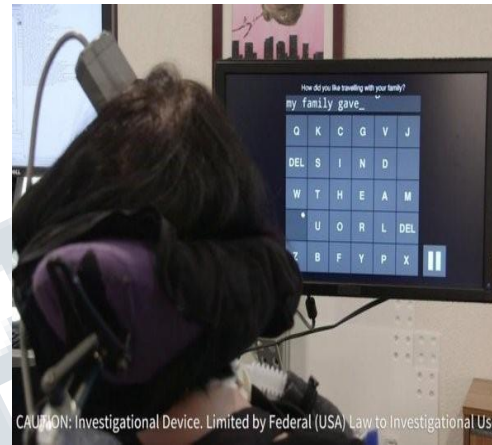
Fig.5: Tetraplegia patient typing words with the help of BCI
