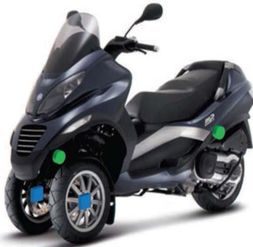
Fig. 1. Test vehicle and sensors set-up. Wheel accelerometers (rectangle), body accelerometers (oval).
