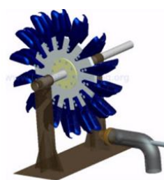
Figure 4: Pelton Wheel Derives Retation From Impulse Force Produced by the Water Jet.
