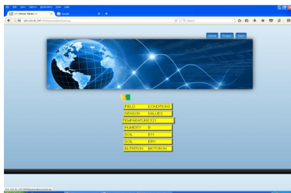
Figure.10: This is the updated page in which the temperature is ranges normal and the Ground level is Dry. Here the MOTOR2 gets "ON".
