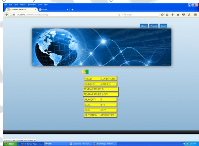
Figure.10: This webpage of the project gets an alert of temperature which is "0". Here the Heating Device to be "ON".
