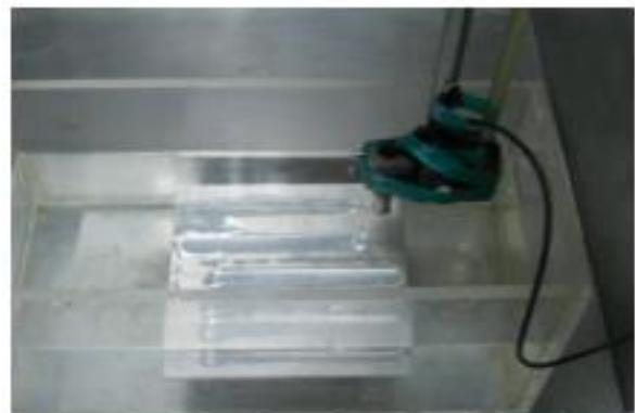
Figure 5: Ultrasonic Immersion Tank
