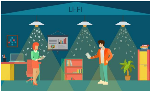
Fig. 1 shows if the light is on then transmit a digital 1 .if it's off transmit a 0 .The LEDs can be switched on and off very quickly which gives nice opportunities for transmitting data
