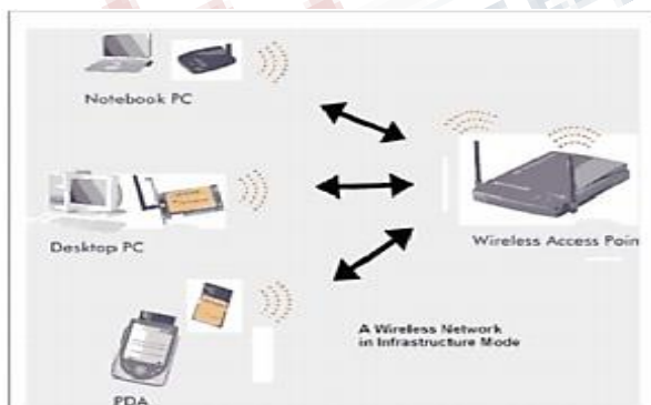
Fig.1 Infrastructure wireless network
