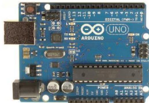
**Fig. 1: Arduino Device**
