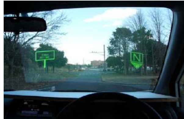
Example of HUD-AR for navigation signs and driving directions projected onto the windshield.
