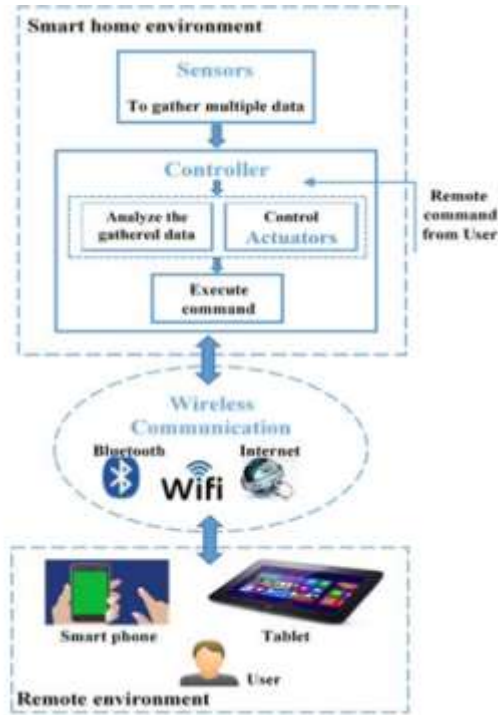
Figure 1: Remote Controlling of the Smart Home
