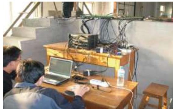
**Figure 1. Strainbook616 data acquisition instrument**
