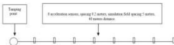
**Figure 2. Arrangement diagram of acceleration sensor horizontal**
