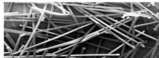
Figure 3: Secondary Electron SEM Image of Nylon Fiber Additions
