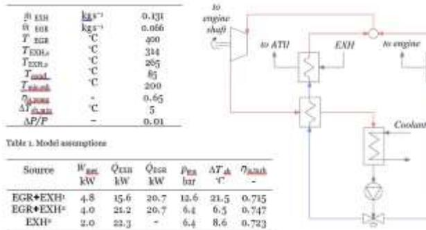
**Figure 1: ORC Component Layout**
