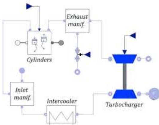
**Figure 2: Object Diagram of the Engine**
