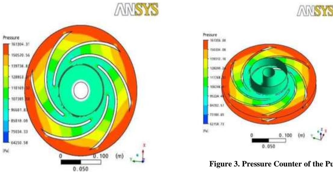
**Figure 3. Pressure Counter of the Pump**
