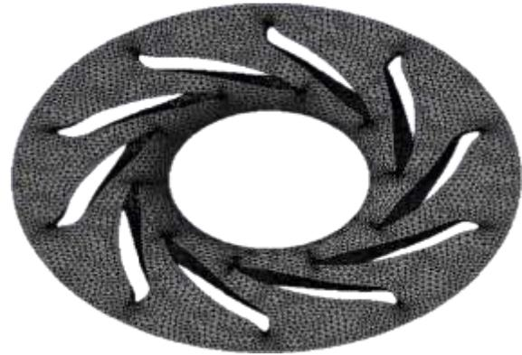
**Figure 1. Meshing Structure**
