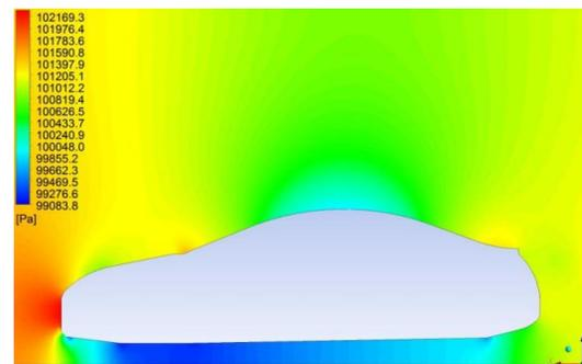
**Fig. 4. Air pressure around the vehicle model**
