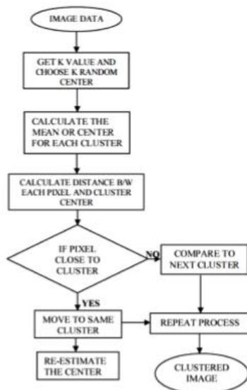
**Fig: Block diagram of K-MEANS method**
