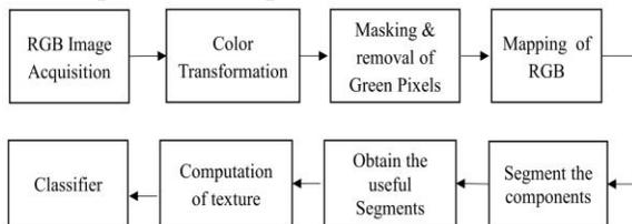
**Fig.** Block Diagram for colour analysis and segmentation
