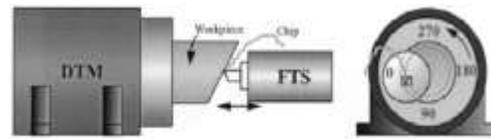
**Fig.3: Experimental Set-up for Fabrication of Tilted Flat Benchmark Test**
