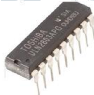
Fig -3: IC ULN2803 APG 500-mA-Rated Collector Current
