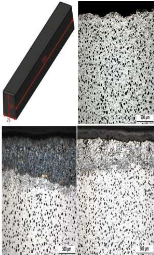
Fig. 1. Produced casting blank geometry (top left), microstructure of EN-GJS-400-15 without rim with surface roughness - PT_III (top right), with rim of lamellar graphite in pearlitic matrix - GE_I (bottom left) and lamellar graphite in ferritic matrix - GE_II (bottom right)
