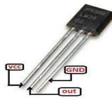
The LM35 –series devices are precision integrated –circuit temperature sensors, with an output voltage linearly proportional to the Centigrade temperature. The LM35 has an advantage over linear temperature sensors calibrated in Kelvin, as the user is not required to subtract a large constant voltage from the output to obtain convenient centigrade scaling. The features of the LM35 make it suitable for many general temperature sensing applications.
