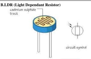
LDR sensor has two cadmium sulphite photoconductive cells (cds) with spectral response to that one of the human eye. The cell resistance will fall with the increasing light intensity. Its applications include smoke detection, automatic lightning control system, and batch counting and burglar alarm systems. Light dependent resistors have property to store the lightning conditions in which they have been stored. Light storage reduces equilibrium time to reach steady state resistance values.
