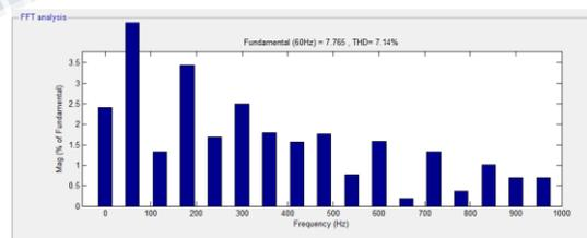
**Fig. 12. THD value of grid current without fuzzy controller at no load.**
