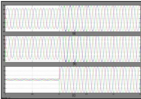
**Fig. 8. iUPQC with fuzzy response at no load condition: (a) grid voltages VA, (b) load voltages VB, and (c) grid currents.**
