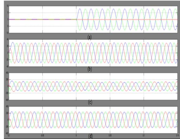
**Fig. 10. iUPQC with fuzzy response during the connection of a two phase diode rectifier: (a) load currents, (b) source currents, (c) load voltages, and (d) source voltages.**
