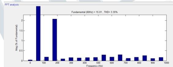
**Fig. 11. THD value of grid current with fuzzy controller at no load.**
