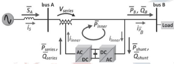
**Fig. 4. iUPQC power flow in steady-state.**
