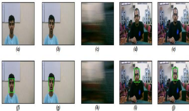
Fig. 11. Detection of Human Faces in a meeting using Audio Sensor Camera – Video Sequence 1 (a) Frame No 13 (b) Frame No 14 (c) Frame No 15 (d) Frame No 16 (e) Frame No 17 (f) Face detection corresponding to Frame No 13 (g) Face detection corresponding to Frame No 14 (h) Face detection corresponding to Frame No 15 (i) Face detection corresponding to Frame No 16 (j) Face detection corresponding to Frame No 17
