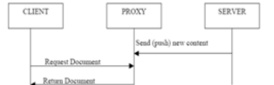
Figure 1: Push technology - A content provider (server) sends new information to proxy and client is notified about it.
