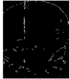
Fig. 9 Cracks obtained by Fuzzy Entropy based Clustering
