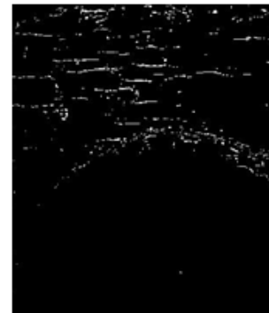
Fig. 19 Cracks obtained by Fuzzy Entropy based Clustering
