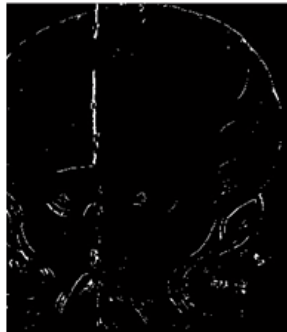
Fig. 7 Cracks obtained by Fuzzy c Means Clustering
