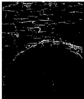
Fig. 15 Cracks obtained by K-Mean Clustering
