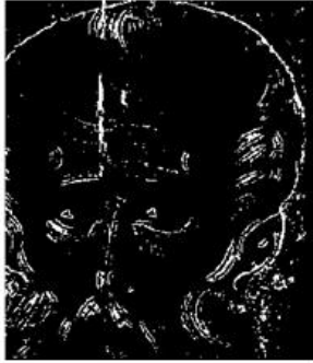
Fig. 5 Cracks obtained by K-Mean Clustering
