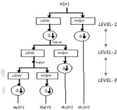
**Fig. 1: Decomposition tree of DWT**
