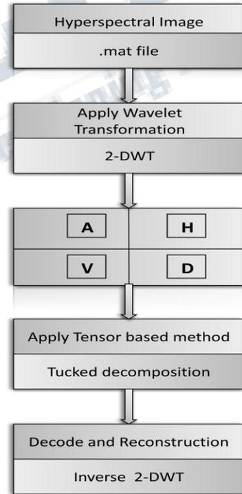
**Fig.4. Proposed System Architecture**
