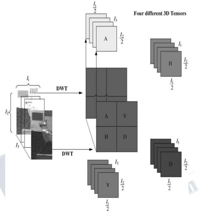
**Fig. 2: Decomposition scheme on the proposed method for HSI.**
