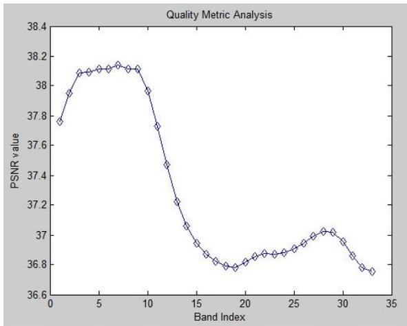
**Fig.6 : Band Index Versus PSNR values for High CR.**
