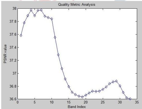
**Fig.7 : Band Index Versus PSNR values for Low CR**
