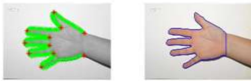
Fig 9 : Two-dimensional hand geometric features marked on a hand for a single sample and Rendered view of the acquired 3-D data.
