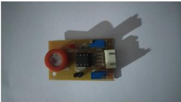
Figure5. CO gas sensor module
