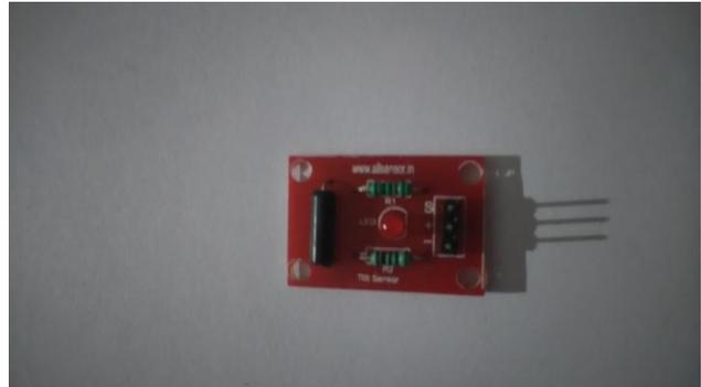
Figure6. Mercury tilt sensor module
