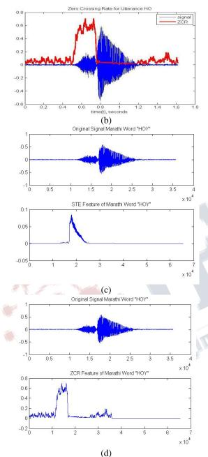
Fig 4. Detection of Speech Non-speech signal using Short time Energy and Zero Crossing Rate (a) and (c) Short time Energy for utterance HOY w.r.t. input signal and (b) and (d) Zero Crossing Rate for utterance HOY w.r.t. input signal.
