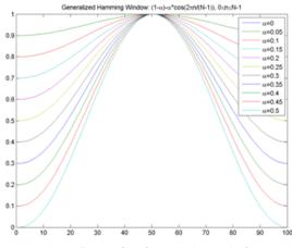
Fig 5. Generalized Hamming Window 3. Fast Fourier Transform
