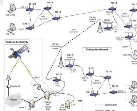
**Figure.1. Configuration for a wireless mesh network**
