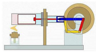
expanded in the hotter portion resulting in a net conversion of heat into work. An internal Regenerative heat exchanger i ncreases the Stirling engine's ther mal efficiency compared to simpler hot air engines lacking this feature.
