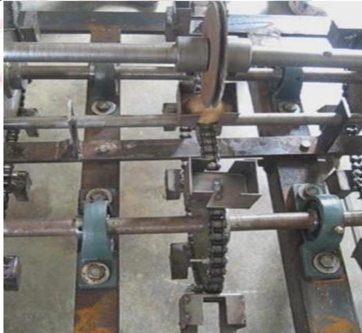
In this experiments a set of two cutters with spacers in-between for each grade of Areca nut were used. The speed of the cutter shaft was at 125 rpm. The Areca nut was fed below the cutters. As it can be seen
