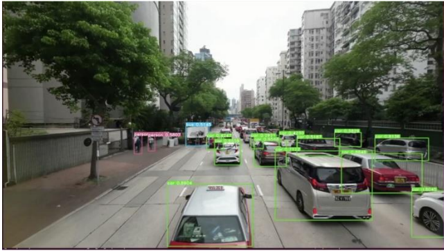
Fig 3 The recognition of the camera for autonomous vehicle sensors
