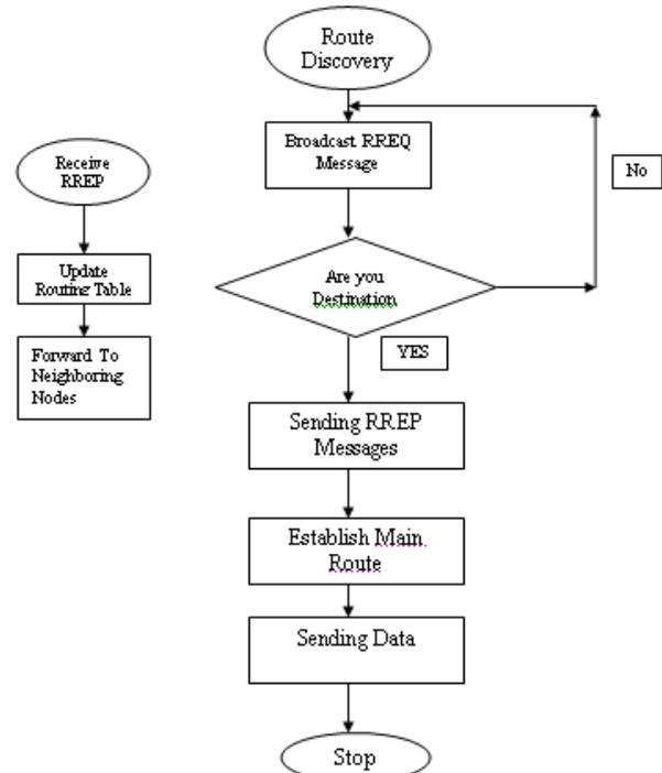
Figure 5: EAOMDV Data Packet Forwarding
